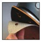
**Caution.** Take care to regularly clean out the build up of dust on the platen undemeath the sandpaper and not to let the sandpaper wear completely down before replacing it. Failure to observe these two precautionary measures can lead to damage to the hooks and loops on the platen and the sandpaper will not attach properly. If the platen is damaged, it can be replaced at an authorised service centre.
